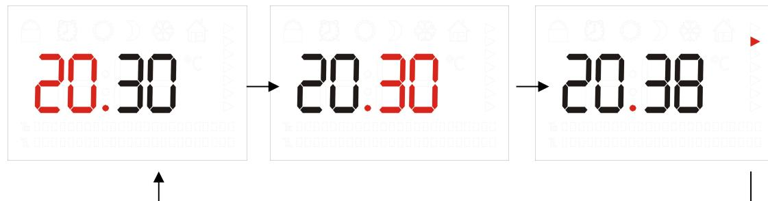
Use the or buttons to modify. After 5 seconds of inactivity the new time is memorised and the program goes back to the CLOCK function.
