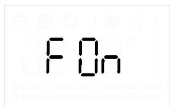
F On: Window Opening detection enabled
