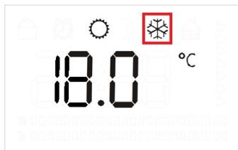
Snow symbol blinking when window open status is detected
